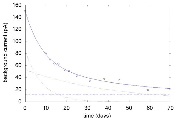
**Fig. 5.** Absolute value of the background current for a charge quantum of 50 fC as a function of time after an integrated X-ray irradiation of 15 kGy: the continuous line shows the function described in Eq. (1) with  $\tau_1 = 8$  days and  $\tau_2 = 41$  days. The dash-dotted line shows the annealing saturation as measured after 1.5 year. Statistical uncertainties are within the dimension of the symbols.
