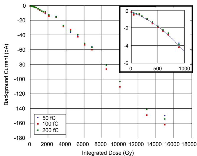
Fig. 3. Background current as a function of the integrated X-ray dose for different charge quanta; the inset shows the trend for doses up to 0.8 kGy. Statistical uncertainties are within the dimension of the symbols.
