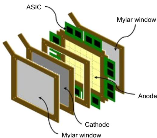
Fig. 1. Exploded view of the pixel detector described in Ref. [10]: the location of the ASICs is shown.
