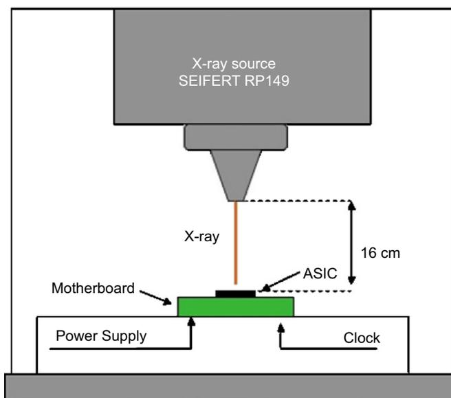
Fig. 2. Sketch of the irradiation setup used at the CERN facility to characterize the ASIC.
